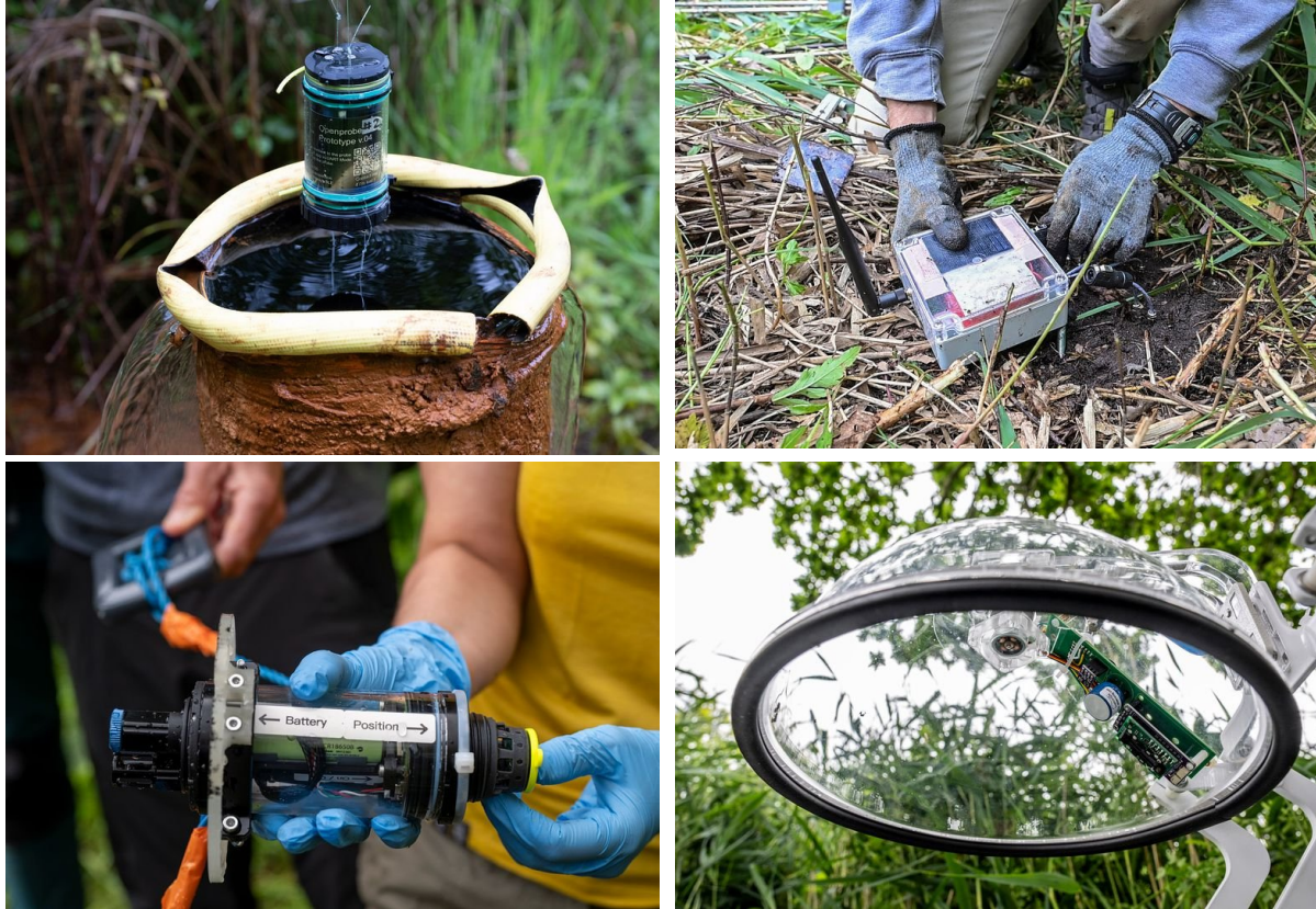
Figure 1 : Developed sensors in-situ during platform deployment on Guidel pilot site (06/2025). From left to right and top to bottom : multiparameter probe, 3 depths soil moisture, water conductivity and temperature measurement system, tracesence passive sampler, transparent Greenhouse Gas Flux Chamber
